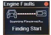
The tool will scan for fault codes from up to four categories depending on the make and model of the test vehicle. It will scan engine faults on all compatible vehicles and optionally scan for Air Conditioning, Auto Gearbox and Ant-lock braking system faults on vehicles with those systems installed and if the appropriate pin is present in the diagnostic connector (See section 4).
